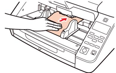
Manual feed mode allows you the option of manually loading sheets of a document for processing.
