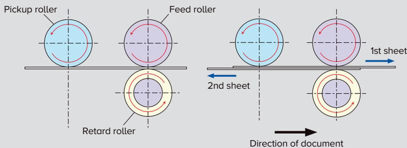
Canon's revolutionary feeding mechanism with retard roller achieves highly reliable page separation.
