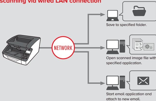
Share a single scanner via a network to perform scanning tasks efficiently. Select any connected computer from the scanner's operation panel and perform scanning. Scanning can also be executed from any computer sharing the scanner
