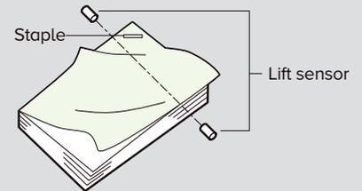
Canon's staple detection feature automatically halts the scanning process if an unremoved staple is found, as staples can cause scanning errors that compromise the document or damage the machine.
